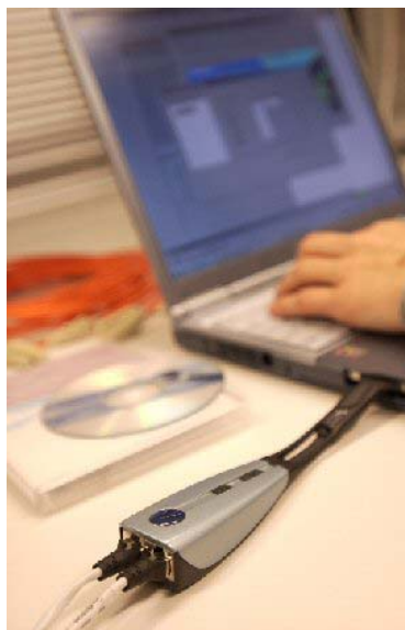
Figure 5: It only takes a few moments to install the NetHawk SS7 Analyser software and plug-in the NetHawk Adapter(s) to the PC. Then your NetHawk SS7 Analyser is ready for use.
