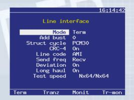
BERcut-E1 provides possibility to perform BER Tests over an entire 2.048 Mbps link using either a G.703 unframed or G.704 framed HDB3/AMI signal. The ability to insert errors in the test pattern, framing and alarm bits allows the user to verify tests and examine error response.
