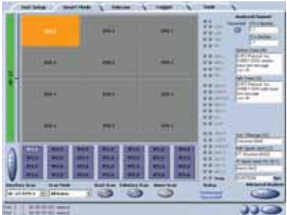
Smart Mode provides automatic discovery of the signal structure of the OC-n/STM-n line, and simultaneously monitors and displays any active alarms and errors on the HO/AU and LO/TU paths, allowing you to easily locate network faults.
