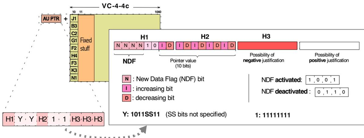
Figure 2 Inside the pointer bytes
