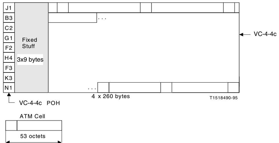
Figure 1 Mapping of ATM cells in VC-4-4c
